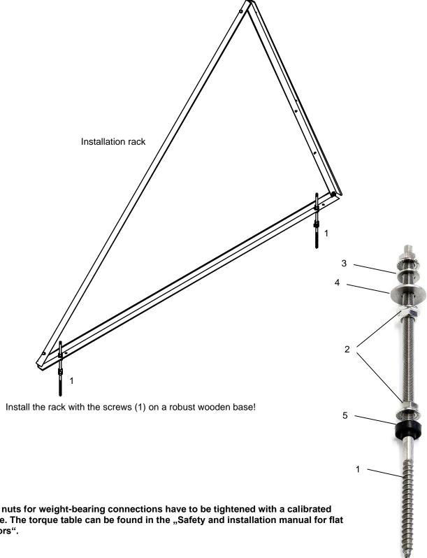
All bolts and nuts for weight-bearing connections have to be tightened with a calibrated torque handle. The torque table can be found in the "Safety and installation manual for flat plate collectors".
