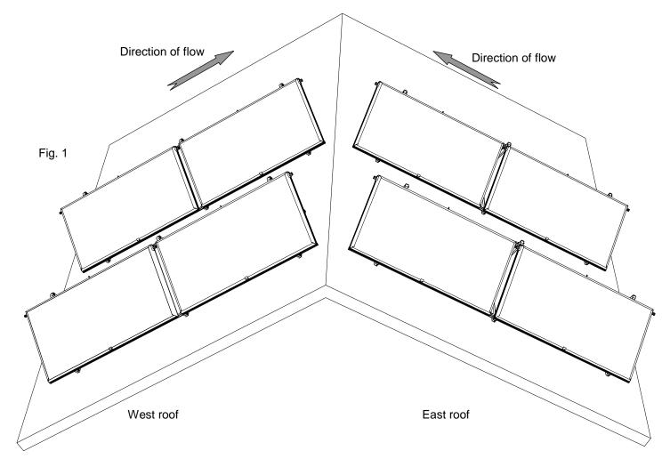
The flow through the collectors has to be from the bottom (eaves gutter) to the top (roof ridge). For West roofs the collectors have to be streamed from the left to the right, for East roofs the have to be streamed from the right to the left.
